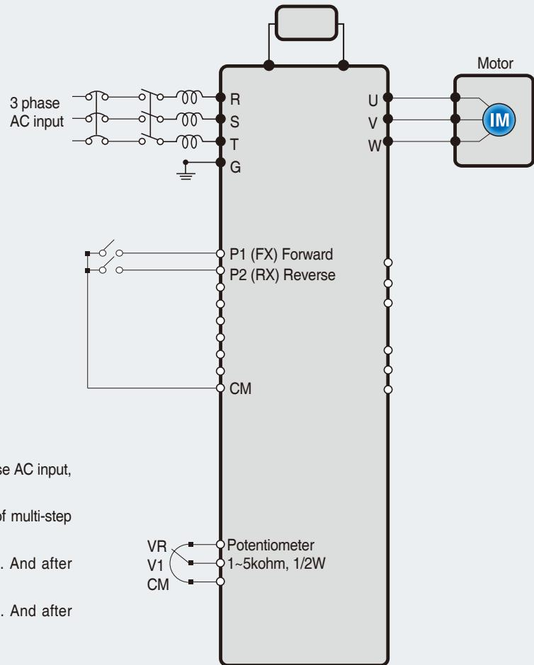
1. Please make sure that R, S, T are connected to 3 phase AC input, and U, V, W are also motor connection terminals.
